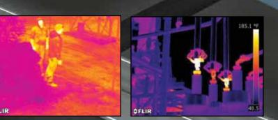
Pole-mounted fixed cameras using FLIR Analytics provide automated alarming of intruders, while cueing pan/tilt cameras to interrogate alarms for more detailed assessment.
